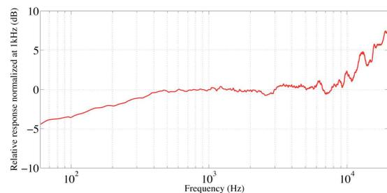
**Figure 5.** PCB mounted MEMS microphone frequency response normalized at 1kHz.
