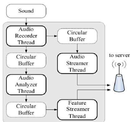
**Figure 8.** Block diagram of Android streamer app.
