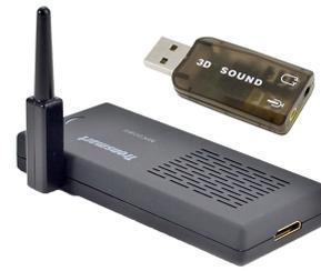
**Figure 3.** Citygram’s Android mini-PC, audio interface solution.
