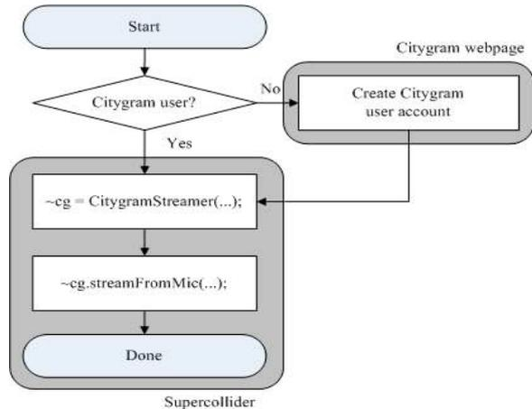
Figure 9. Streaming setup in Supercollider.
