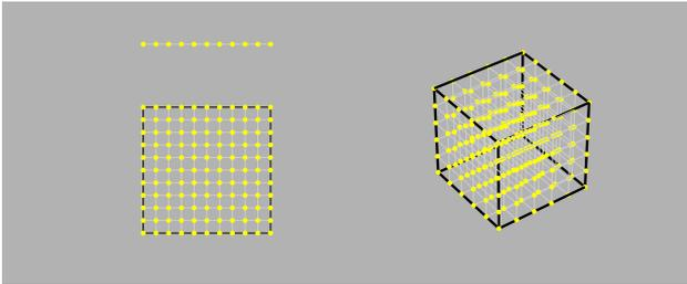
**Figure 2.** Regular grids used in the solution of systems in 1D, 2D and 3D.
