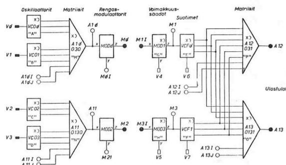
**Figure 2:** Block diagram of the DIMI-6000 signal path [5]
