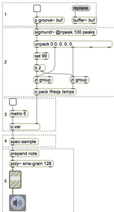
**Figure 6:** A granular synthesizer that chooses the frequency of each grain from a spectrum produced by sigmund~ using the amplitudes of each frequency component as a probability distribution.
