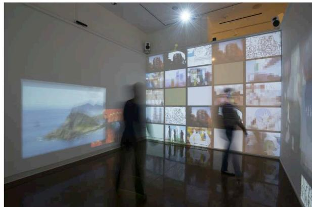
**Figure 1.** This photo shows two people moving through the *Time Jitters* installation. Three of the four walls are visible. The left-most and right-most walls are interactive. Also visible is one of the two Kinects used in the installation (top left), two of the four speakers, and one of the four projectors.
