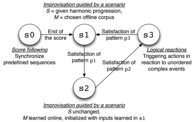
Figure 4. Schematic example of an improvisation plan.
