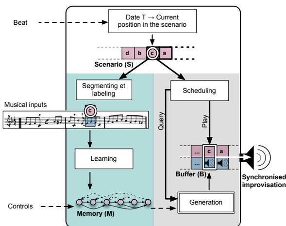
**Figure 2.** The generation process within a real-time architecture.
