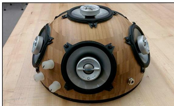
Figure 5b. 6-channel hemispherical speaker
