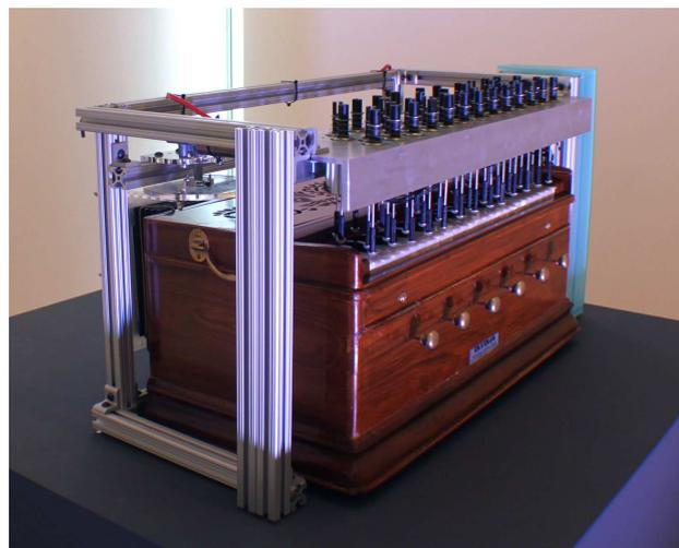
**Figure 1.** Kritaanjli. Shown in this image is Kritaanjli's chassis and attached actuators.
