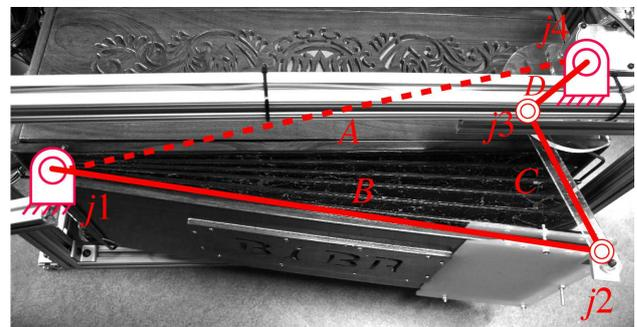
**Figure 5.** Kritaanjli's four-bar linkage bellows-pumping mechanism. The crank is visible on the image's right; the rocker (the hinged harmonium bellows) is on the image's left. Overlaid on the image is a drawing of the assembly's elements.
