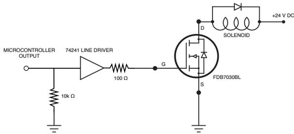
**Figure 9.** Kritaanjli’s solenoid circuit. A line driver is used to allow for longer cable runs between the microcontroller and the Persephone board. The same circuit is used for Kritaanjli’s bellows pumping motor.
