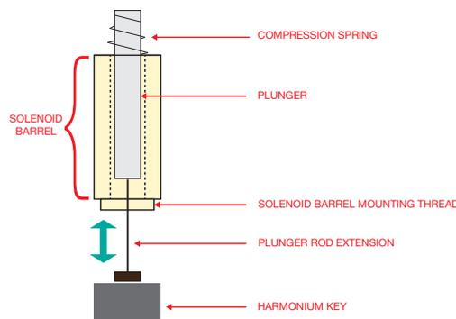
**Figure 4.** A drawing of one of Kritaanjli’s solenoid actuators. Upon actuation, the plunger is drawn fully into the solenoid barrel and the rod extension is pressed against the harmonium key. Upon deactivation, the compression spring pulls the plunger from the body.
