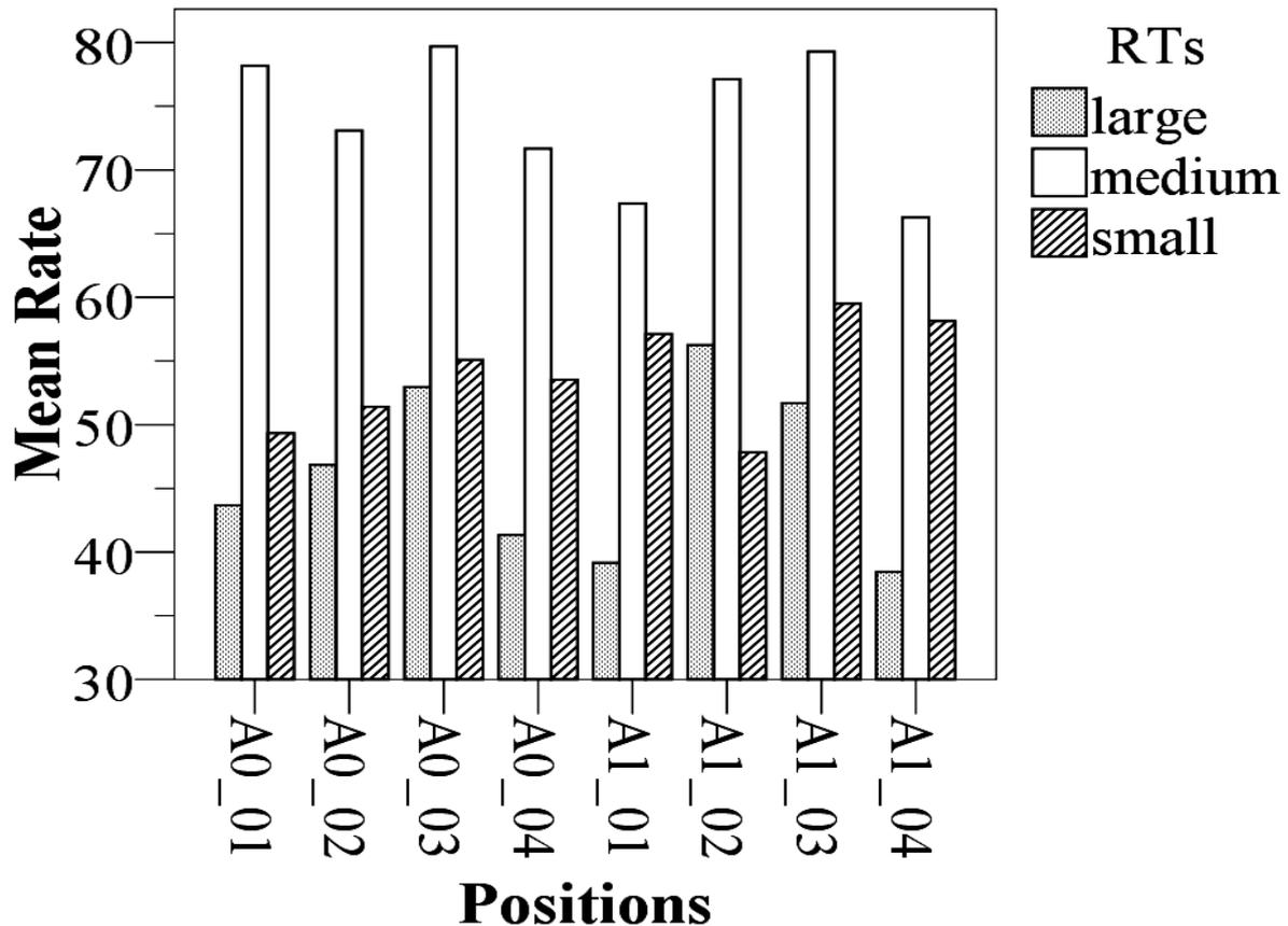
Figure 7. Rating of reverberation preference, as function of different source / receiver position and church size.
