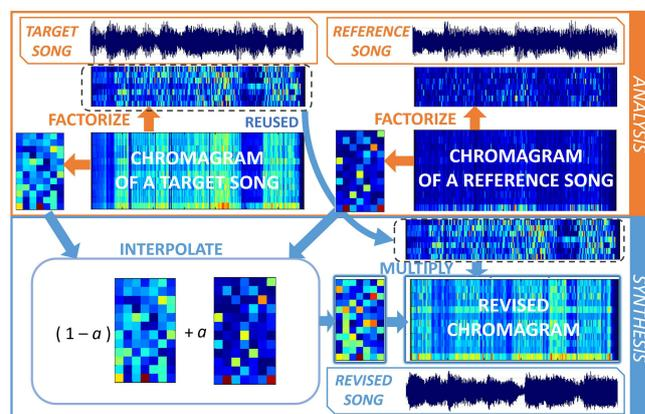
**Figure 1.** Process flow of *HarmonyMixer* mixing the character of chords among polyphonic audio. The method factorizes a matrix consisting of chroma vectors, interpolates the bases obtained through the factorization, and converts the spectrum to create an audible modification in the chords.
