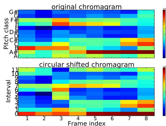
**Figure 2.** Example of chromagram and its circular shifted chromagram. It is created by a circular shift as whose maximum value within a chroma vector to be the first element (interval=0). With this feature, typical chord types are observed removing the transposition of chord driven by the change of the root note.
