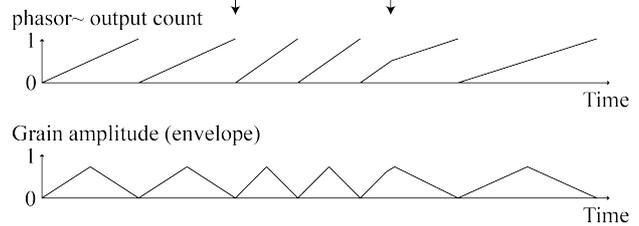
**Figure 1.** Control of grain envelopes from a phasor~ object. Arrows point user-changed parameters for period, which may happen during a ramp and are taking effect immediately. No delay is possible between successive grains.
