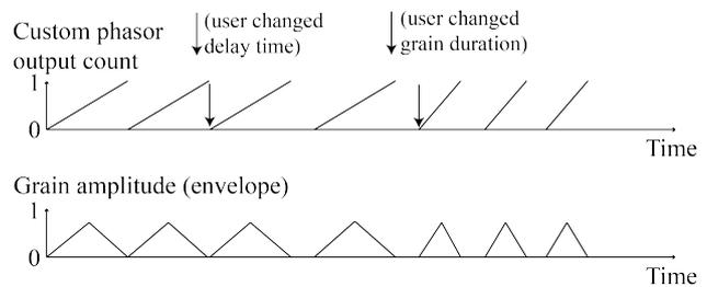
**Figure 2.** Control of grain envelopes from a custom phasor object. Top-level arrows point user-changed parameters for pseudo-period (duration and/or delay time). Bottom-level arrows point the time at which the parameter change actually takes effect, at the beginning of each pseudo-period. Delay is possible between grains.
