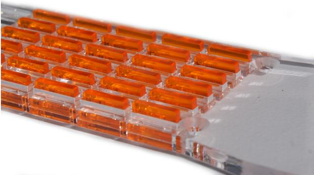
**Figure 8.** First version of the BLADEAXE laser cut acrylic buttons.
