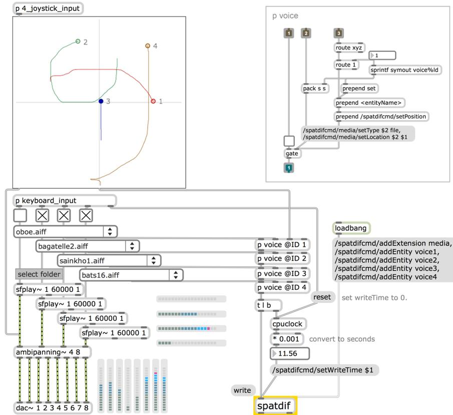
**Figure 4:** MaxMSP implementation, demonstrating the recording of four manually generated trajectories obtained from joysticks. The upper right shows the ‘voice’ section responsible for formatting the media and position inputs.
