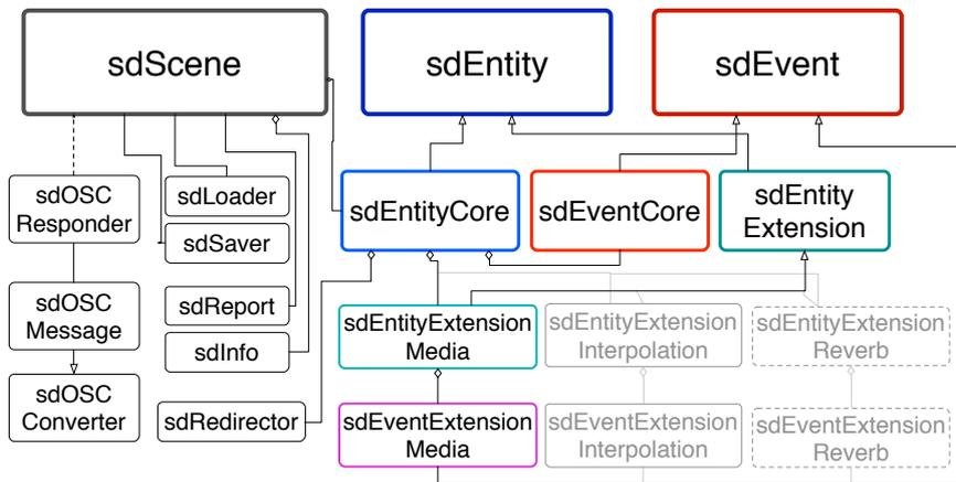
**Figure 2:** Simplified class hierarchy of the SpatDIF software library. The top row shows the three main classes, below are the derived subclasses coloured according to their parents. The interfacing and utility classes are located on the left and future extensions on the right are marked in grey.
