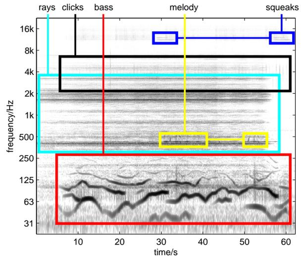
**Figure 3.** Spectrogram of stimulus 2 based on transformation with logarithmic frequency resolution (short-term constant Q transform, ST-CQT [13]). Sound objects of Tab. 2 largely cover distinct frequency bands (colored boxes).
