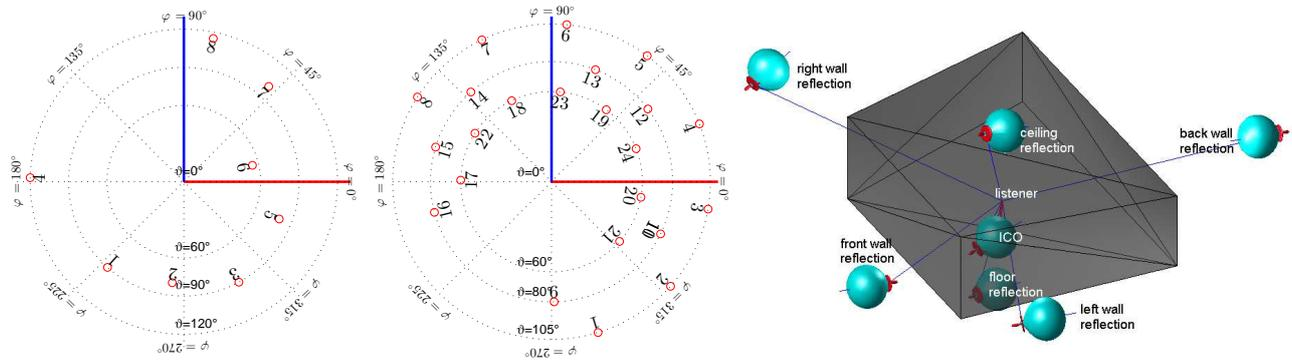
**Figure 2.** Layouts of the pieces *grrawe* (left) and *firniss* (middle) in terms of beams (see numbers) to which the composition routes and amplitude-pans its signal objects. The image on the right shows the mirror sources representing wall reflections of the ICO, cf. Tab. 1, including an exemplary beam pattern pointing at the back-wall reflection.
