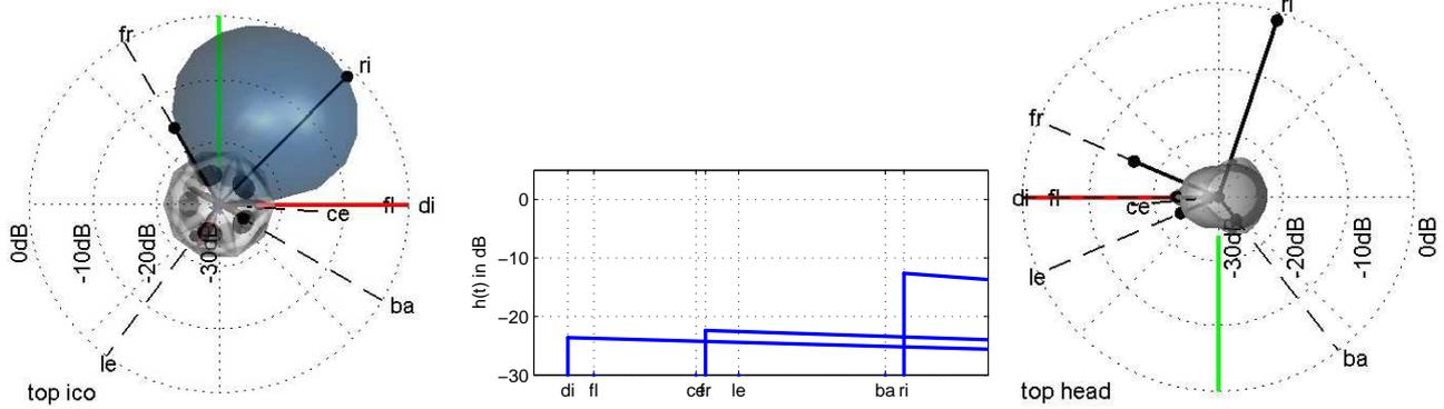
**Figure 4.** Reflection paths as they are excited by the stimulus example *squeaks* through the ICO are shown in the polar top view (left). Time sequence of arriving reflections at the listener and their *echo thresholds* are shown in the middle. The polar top view on the listener (right) shows from where reflections arrive with which propagation decay.
