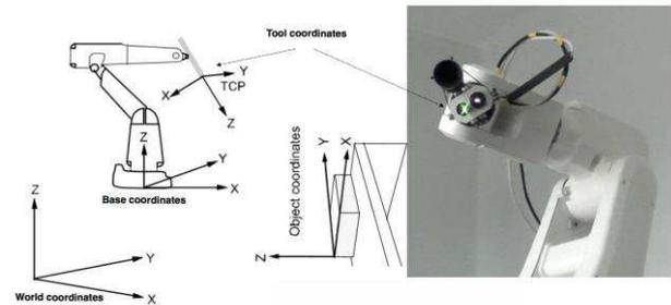
Figure 6: The orientation of the x,y,z axis for the robot tool and the work object,.
