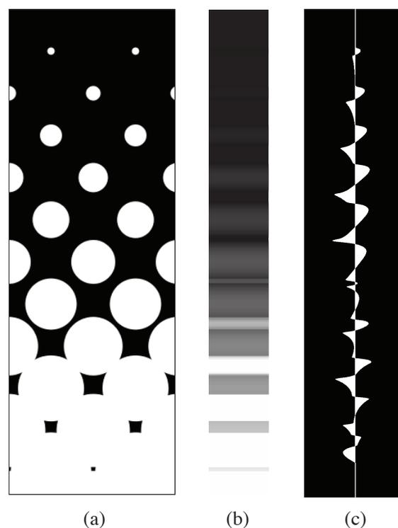
**Figure 3.** Depiction of the optical sonification process: the lightness values of the source frame (a) are averaged to return a column of values (b), which are then filtered and multiplied by a scalar to produce the waveform (c)
