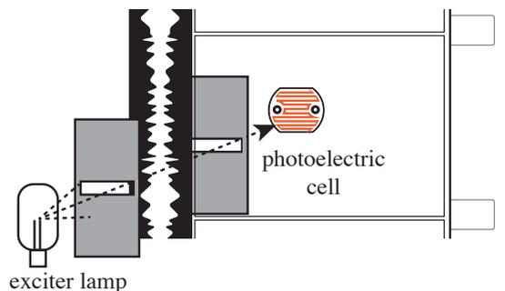
**Figure 1.** Diagram of the optical sound head
