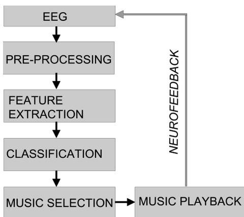
Figure 3. Diagram of the BCI neurofeedback system.
