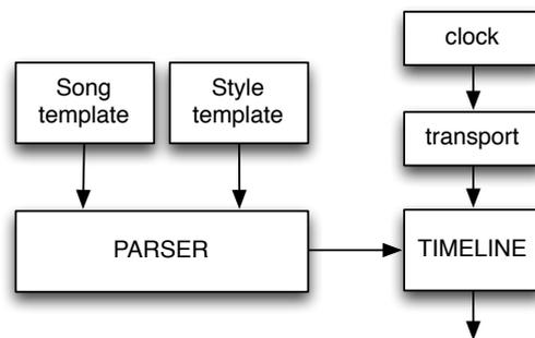
Figure 9 Sequencer structure
