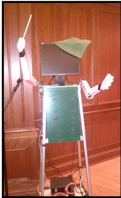
Figure 1. Conducting humanoid robot Link.
