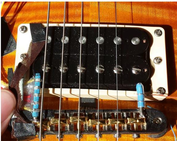
**Figure 6.** Pressure sensor soldered on the saddle of a Les Paul bridge, sensing palm pressure along the string.
