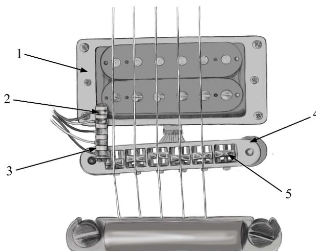
**Figure 1.** Diagram of the developed pressure sensor and its disposition: (1) Pickup; (2) Conductive band; (3) Fret (used as a sensor support); (4) Bridge; (5) Saddle.
