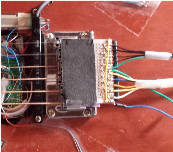
**Figure 2.** First attempt to sense the guitar thanks to a pressure sensor array attached right onto the guitar bridge.
